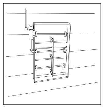
Figure 4-4 Movable Louvers For Air Inlet
